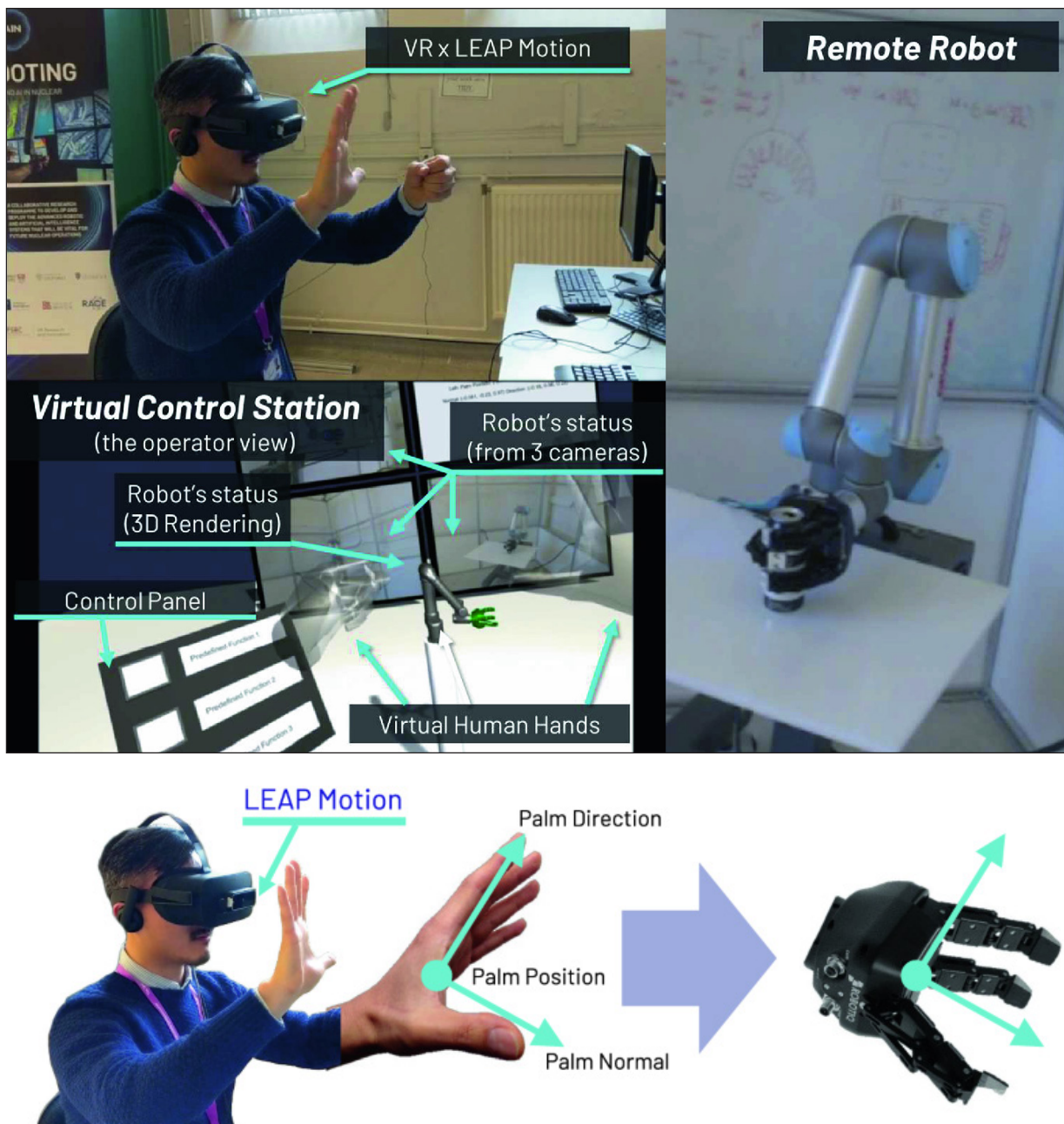
Figure 13: Example of system combining ROS to Unity3D for Virtual Reality and remote control
