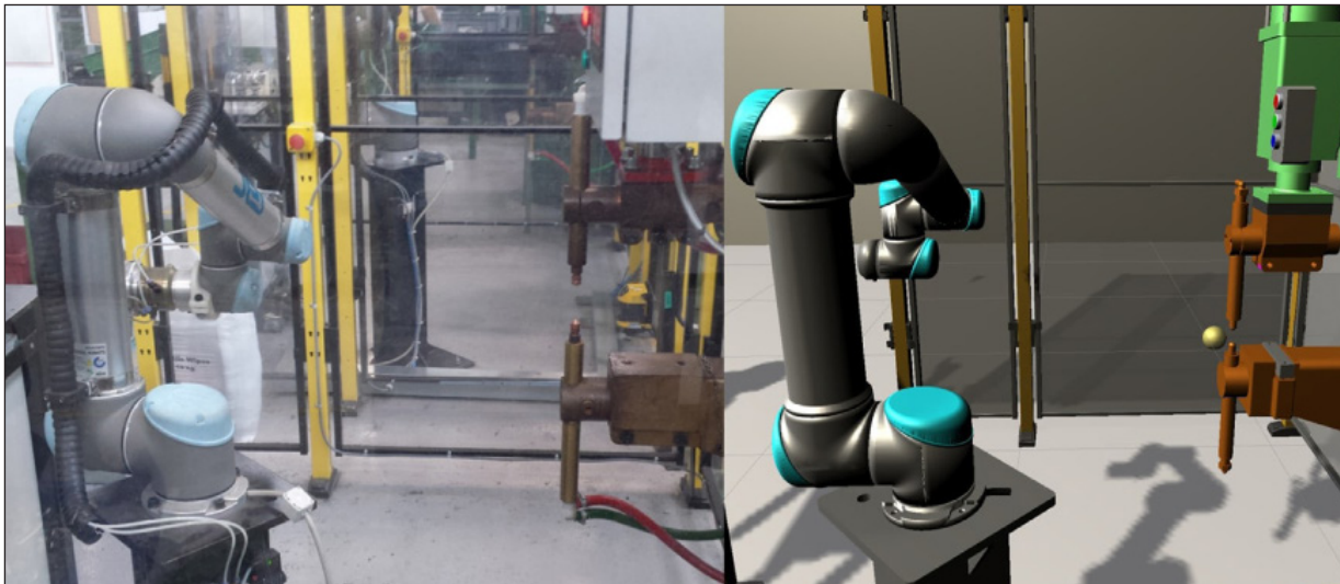
Figure 4 : A side by side view of the physical and digital twins in real-world industrial welding process.
